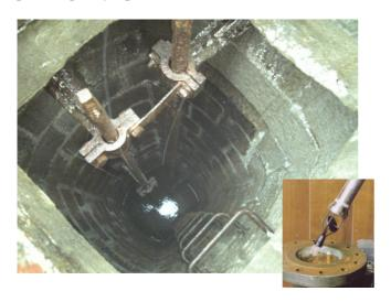
BAHS down hole CCTV equipment has a 350 metre umbilical cable rated to operate at depths of up to 300 metres below the water level.
