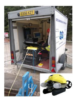
BAHS are pleased to present a new remote operated vehicle (ROV) for use within tunnel and adit inspections. The versatile Videoray Pro 4 has a depth range of ~300 metres and a lateral range of up to 400 metres. For surveys of greater distances BAHS are able to arrange ROVs capable of up to 1,500 metres.
